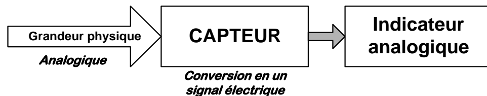
Figure 1.1: Block diagram of an analog measurement system.
